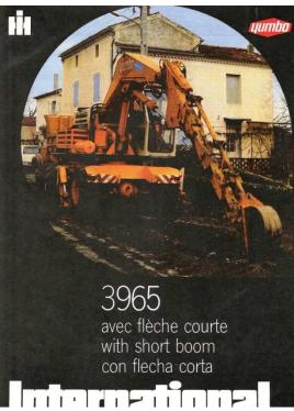
Carlo and Mario Bruneri of Italy. This was the first fully hydraulic excavator and Yumbo or SICAM (Society de Industrial Construction of Mechanical Hydraulic Appliances) bought the patent rights in 1954. Some say the Gradall of 1941 was the first hydraulic excavator built in Ohio. This was built a little different than the Yumbo with a boom that moved in and out. It was also mounted on a truck. A lot of
